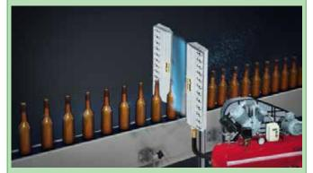
Two (2) **Model AE12SDS-1** Stainless Steel (Type 303) Regular Air Knives are used to blow-off liquid from one liter soda bottles. The elimination of the water on the bottle allows the labels to properly adhere. Before the Air Knives were installed, the customer estimated that they wasted 3%-5% of their labels. The cost savings multiplied over thousands of bottles was significant.
