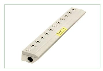
The Advanced Air Knife is an eco-friendly and energy efficient way to clean, cool and dry applications. Without using any electricity or any moving parts, the Advanced Air Knife produces a high velocity, high flow laminar sheet of air by using only a small amount of compressed air as its power source. The Advanced Air Knife provides an amplification ratio of 40:1 and air consumption of 2.9 SCFM per inch at 80 PSIG.
