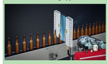
Two (2) **Model AE12SDS-1** Stainless Steel (Type 303) Regular Air Knives are used to blow-off liquid from 1 Litre soda bottles. With the elimination of water, the labels are now able to properly adhere. Before installation of the Air Knives, customer estimated they wasted 3 - 5% of their labels. At thousands of bottles per day, this cost can quickly add up.
