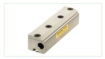
Streamtek's Regular Air Knife offers a more efficient and eco-friendly way to provide superior quality cleaning, drying, cooling, heating and decontaminating for any application. The Regular Air Knife produces an even laminar flow of air that turns 90 degrees through its entire length at an amplification ratio of 30:1 and air consumption of ~3.4 SCFM per inch at 80 PSIG. Our Air Knives are made from Aluminum or Stainless Steel material.
