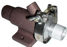
Consist of a VT Vacuum Transducer and a Cap. An example of a complete part number could be a VT750C1. The VT750 indicates an "A" diameter of .750". The C1 Cap also has a .750" diameter with a 3/4" NPT thread. Cap part numbers C1-320 through C1-750 have 3/4" NPT threads and the C1-940 has a 1" NPT thread.
